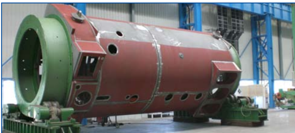
The outer casing of the generator is currently under construction at a Siemens subcontractor in Hungary.
