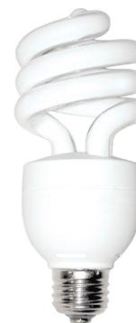
In fluorescent lights, a current is passed through mercury vapour to produce ultra-violet energy. A fluorescent powder coating placed inside the tube absorbs the ultra-violet energy and, in turn, glows and gives off visible light. In both incandescent and fluorescent lamps only a small amount of energy is turned into light – the rest is converted into heat energy.
