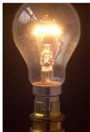
The simplest method of converting electrical energy to light energy is with a filament lamp. Filament refers to the special high resistance wire (usually tungsten) used inside the bulb, which can be drawn into very thin wires that does not melt even when heated to about 2600°C.
