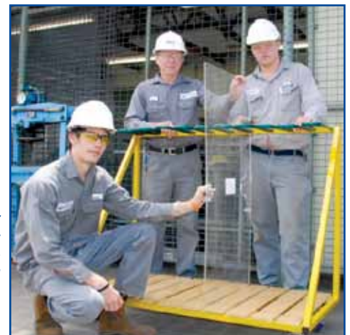
GSESC students Ben Thomas and Brendan Crawford and teacher Peter Hamment inspect the new acrylic door rack which will allow the safe storage of 6.6kV protective shields.
