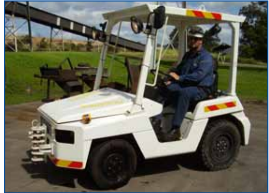
Kurt Roberts checks out the new tow tug which will be used to remove pulveriser rotors.
