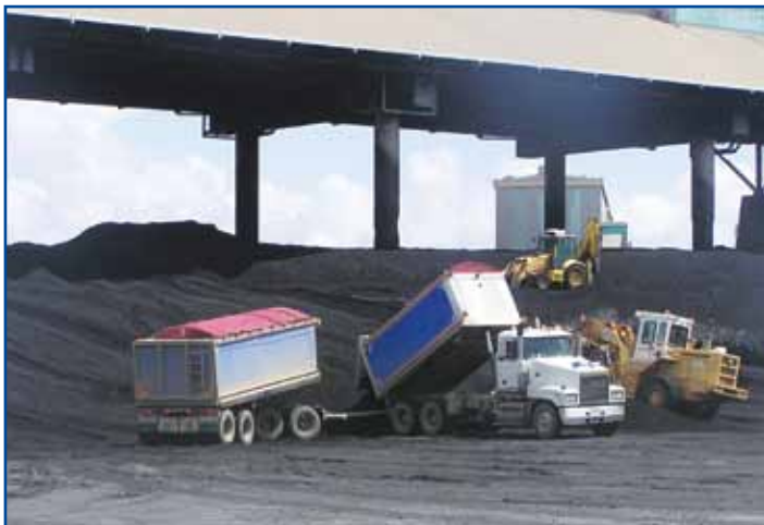
Coal from RG Tanner Terminal is unloaded at the coal plant slot bunker.
