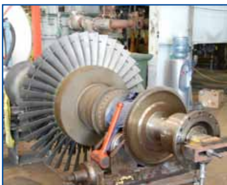
The boiler feed pump rotor ready for inspections.
